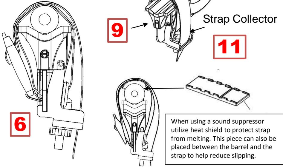
**Disclaimer:** The bayo is designed to fit tapered and bull barrel muzzles between 0.50 and 2.00 inches in diameter. It is the responsibility of the user to make sure that the bayo is mounted correctly with the sensor deck away from the bullet path. It is the user's responsibility to monitor the tightness of the strap as some loosening can be experienced on some weapons. Failure to do this could result in damage to the unit or serious bodily injury!!
