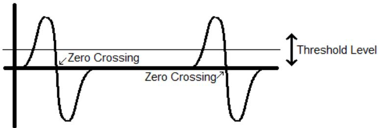
Sketch of the signal from a standard copper-jacketed, lead bullet.
